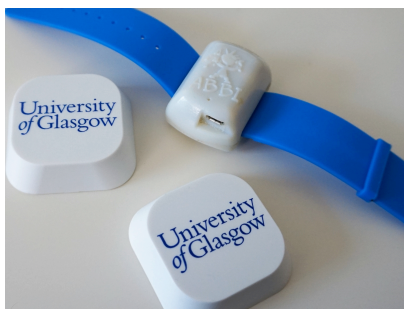
Figure 1: ABBI bracelet prototype and two of the kontakt.io beacons used by our system. Future iterations of the bracelet will have a smaller and more appealing design for children.
