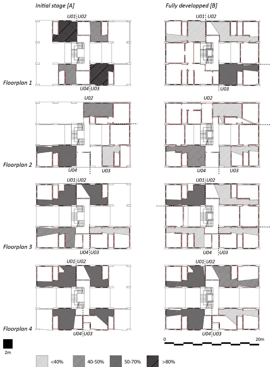
FIGURE 8. 360° isovist polygon drawn from a location inside the unit in front of the entrance door. The percentage of area taken by the isovist polygon on the overall area of the unit.
