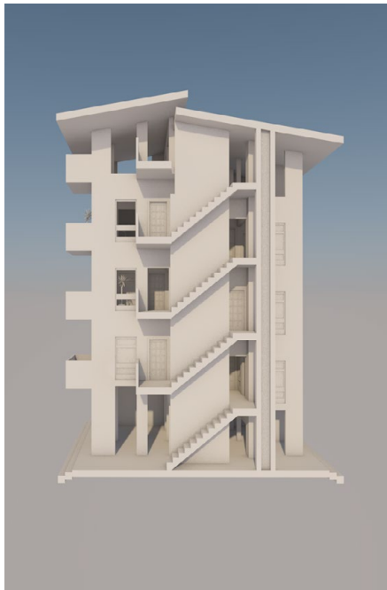
FIGURE 10. Typology in the design proposal (Incremental Building 2): the building is design to reproduce the spatial configuration of the traditional Malaysian houses (level distinction, double entrance , open yards) in a more dense apartment block.
