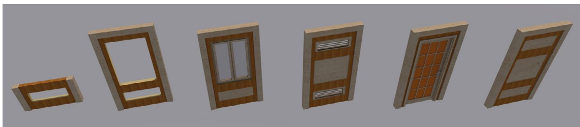
FIGURE 7. Modularity and demountability in the design proposal (Incremental Building 1): elements are designed to implement a structure-infill approach, to increase flexibility and to facilitate self-construction for non-structural parts of the building
