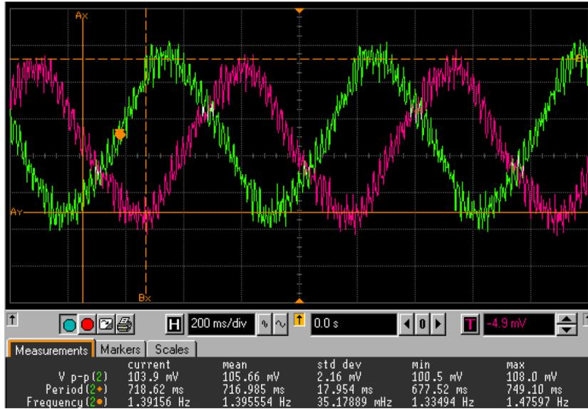
Figure 6: Oscillograms of the recorded steady-state currents in two phases of the shorted secondary winding for the unloaded BDFRG at  $\approx 730$  rev/min.
