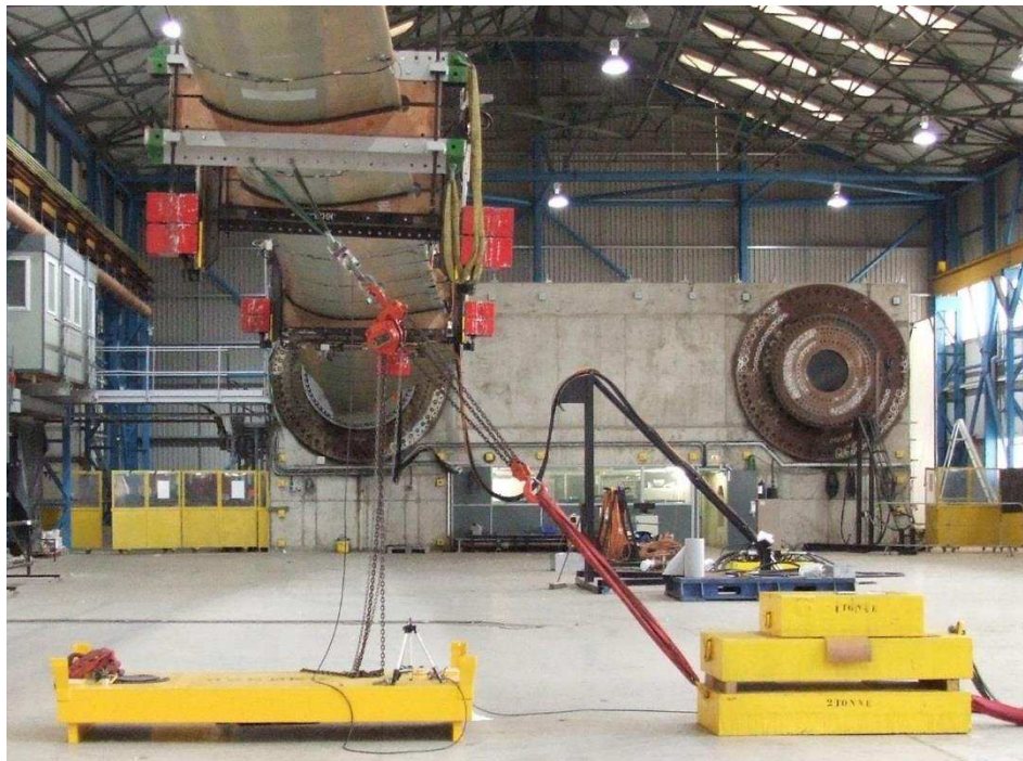
Figure 4. Combined load test configuration
