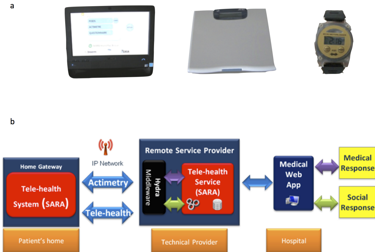
Figure 1. inCASA platform elements: (a) patient's equipment (computer, scale, and actigraph); (b) information system technical architecture.
