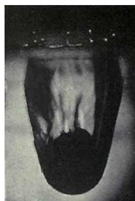
Figure 6: Figure from Worthington [4] which shows the cavity formation at the wake of a rough sphere following its water entry. The sphere had a diameter of 1.5cm and was released from a height of 15cm.
