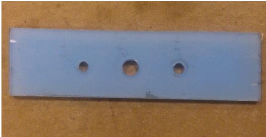
Figure 9: A plastic piece used to hold the spheres in place prior to their release. The centre hole was the place where spheres were placed and had the same diameter as the spheres. The two smaller holes at either side of the centre hole was used for the screws to attach the plastic piece to the electromagnet.
