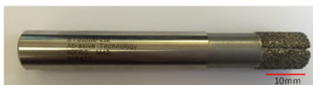
Figure 9. Unused diamond bonded 10 mm diameter end mill.
