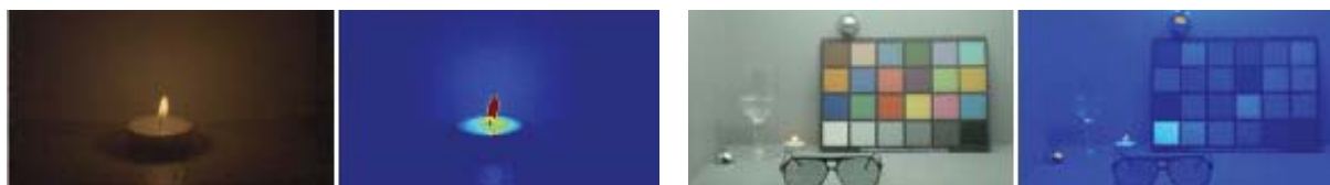
Fig. 1. A single candle lit in dark a room has a dynamic range 16.8 million to 1, while items evenly lit by sunlight only have a dynamic range of 256 to 1 (Image courtesy of Jassim Happa).
