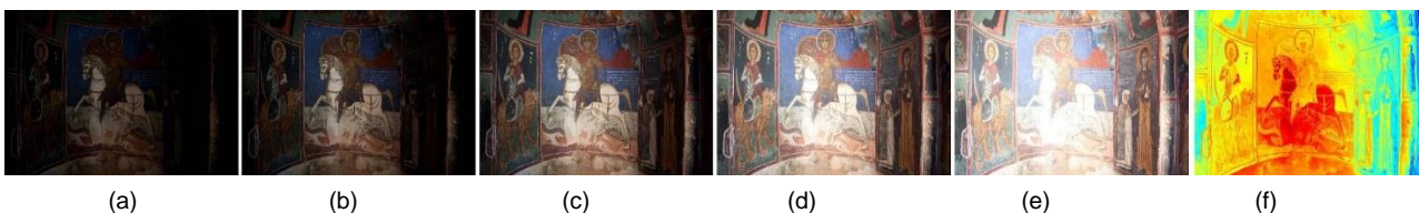
Figure 2: Asinou Church fresco captured with the bracketing technique. The exposures are: a) -2 EV; b) -1 EV; c) 0 EV; d) +1EV; e) +2EV. The last image f) is the result of the merged luminance values represented in false colours, the false colours technique allows the range of lighting in an HDR image to be visualised on a non HDR display.
