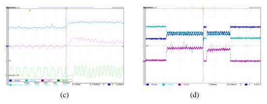
Figure 6.9: Mode detection (Y axis: 1 A/Div for i1 and i2, 2 V/Div for Vc, and 5 V/Div for PWM): (a) mode change without detection (X axis: 40 ms/Div), (b) mode change with detection (X axis: 200 ms/Div), (c) mode change with detection (X axis: 1 ms/Div), (d) mode change with 100 ms CFC off time (X axis: 400 ms/Div).
