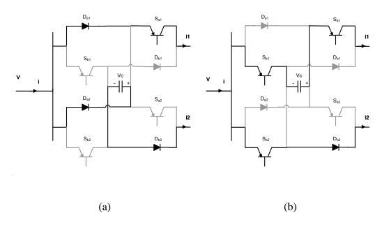
Figure A.30 Reduced switches count topology MCFC operating in mode 2. a) Charging period, b) discharging period.
