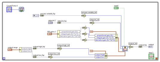
Figure C.5 LABVIEW PID controller loop.
