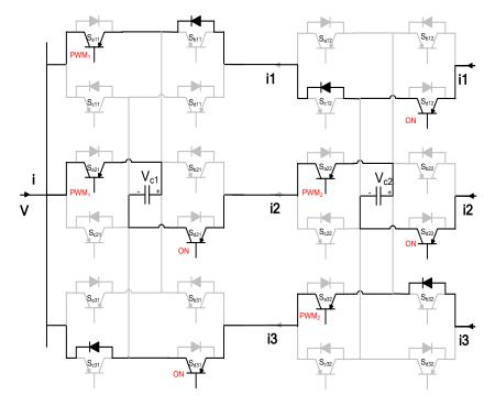
Figure A.28 Three ports MCFC operating in mode 6 - reverse (discharging period).
