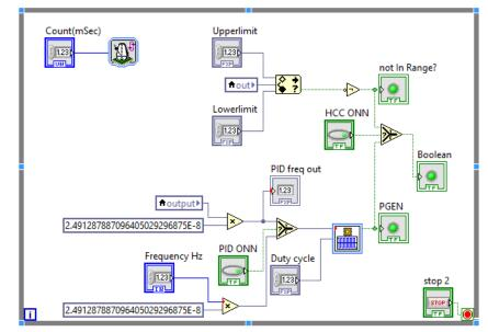
Figure C.6 LABVIEW controller selection loop.
