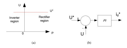
Figure 3.2: Operation in constant voltage mode a) DC terminal voltage Vs power characteristics. (b) Controller schematic.
