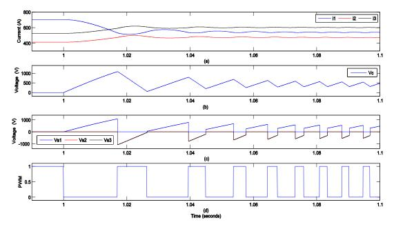
Figure 4.39 Extended CFC unsuccessful balancing (mode 1) - extended topology. (a) Cable currents, (b) Capacitor voltage, (c) Series voltages, (d) PWM signal.
