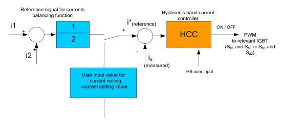
Figure 4.12 Proposed Hysteresis band current controller for CFC.
