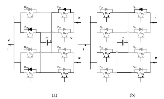
Figure 4.6 CFC operating in mode 3 (reverse). (a) Charging from cable 1. (b) Discharging in cable 2.
