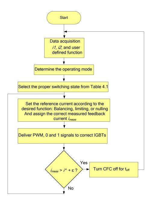
Figure 4.15 Flow chart for automatic mode detection and change algorithm.
