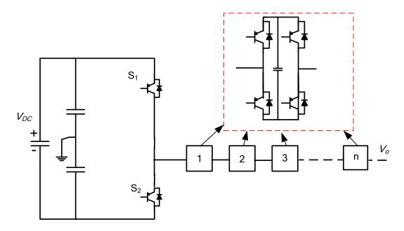
Figure 2.12: Hybrid H-bridge cascaded multilevel converter.
