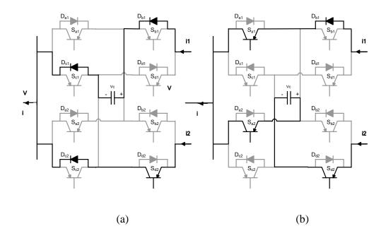
Figure A.3 Two port CFC in in mode 3 (reverse). (a) Charging from cable 1. (b) Discharging in cable 2.
