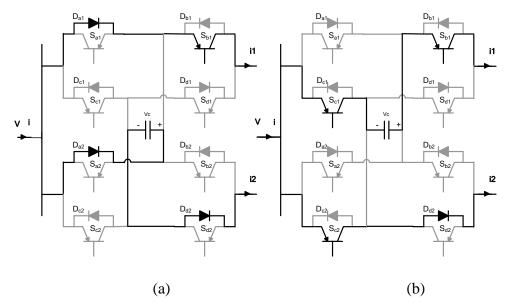
Figure A.2 Two port CFC in in mode 2. (a) Charging from cable 2. (b) Discharging in cable 1.
