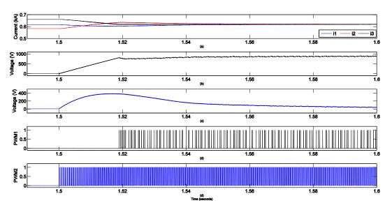
Figure 5.11 MCFC currents balancing - mode 3. (a) Cable currents, (b) Capacitor voltage *V*<sub>*c*1</sub>, (c) Capacitor voltage *V*<sub>*c*2</sub>, (d) PWM<sub>1</sub> signal, (e) PWM<sub>2</sub> signal.
