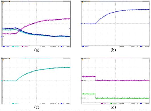
Figure 6.14: Nulling i1and i2 – MCFC (Y axis: 1 A/Div for i1, i2, and i3, 5 V/Div for Vc, and 5 V/Div for PWM, X axis: 4 ms/Div): (a) cable currents, (b) capacitor voltage Vc1, (c) capacitor voltage Vc2, (d) PWM signals P1 and P2.
