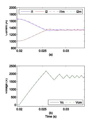
Figure 4.45 Comparison between simulation and calculation results (a) Cable currents, (b) Capacitor voltage.
