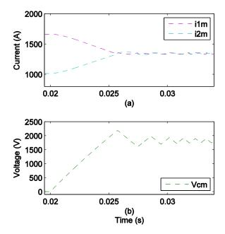
Figure 4.44 Calculated mathematical model outputs (a) Cable currents, (b) Capacitor voltage
