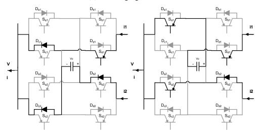
(a) (b) Figure A.4 Two port CFC in mode 4 (reverse). (a) Charging from cable 2. Discharging in cable 1.
