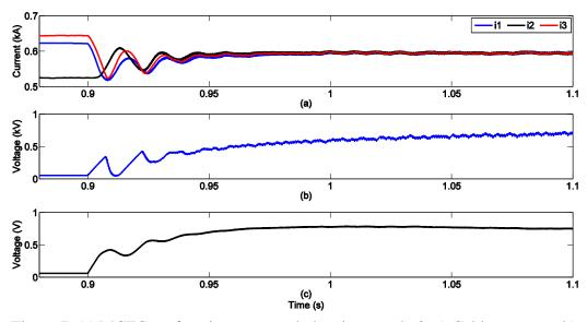
Figure B.11 MCFC performing currents balancing: mode 3. a) Cable currents, b) Capacitor voltage Vc1, c) Capacitor voltage Vc2
