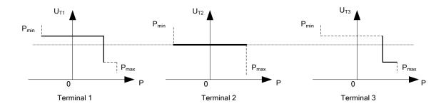
Figure 3.3: DC terminal voltage Vs power characteristics of a three terminals grid with voltage margin control.
