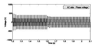
Figure 3.14: Phase to Phase voltage VAB at the AC side of the converter.
