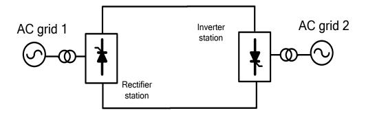
Figure 2.3: Back to back LCC based HVDC system.
