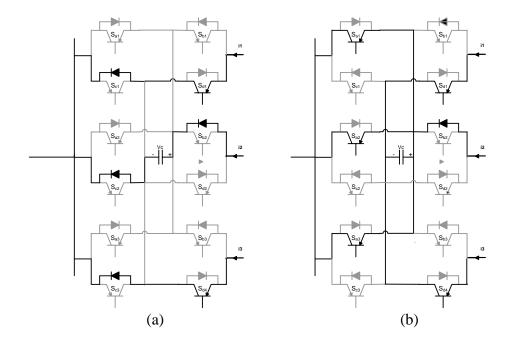
Figure A.12 Extended CFC mode 8 (reverse) a) Charging from cable 2, b) Discharging in cables 1 and 3.
