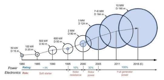
Figure 1.2 Evolution of wind turbine diameter length and it's power electronics [15].
