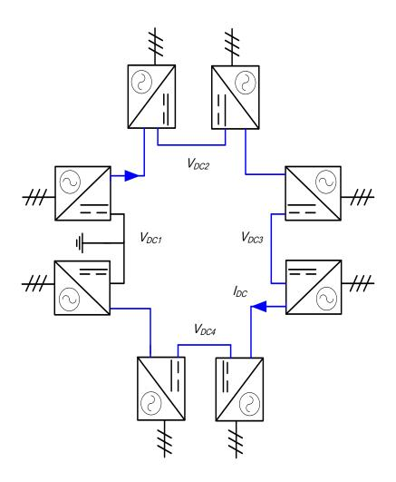
Figure 2.18: Series bipolar MTDC connection.
