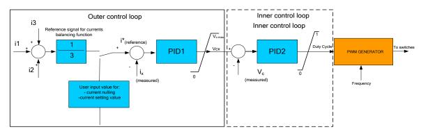
Figure 4.19 Proposed PID control scheme for the extended 3 ports CFC.
