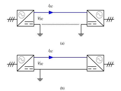
Figure 2.15: Monopolar HVDC point to point connection a) Ground return b) metallic return.
