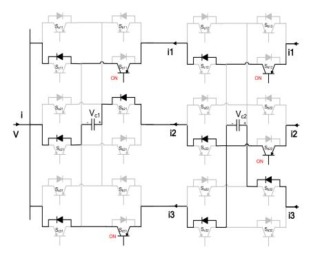
Figure A.25 Three ports MCFC operating in mode 5 - reverse (charging period).
