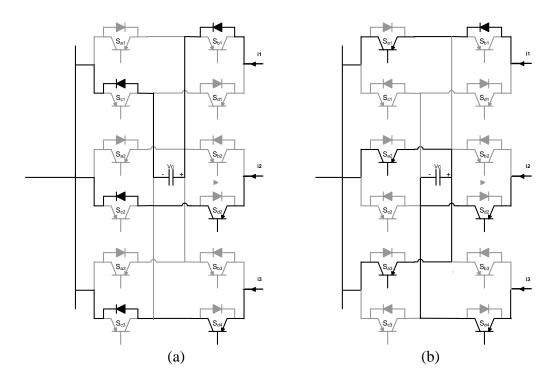
Figure A.11 Extended CFC m ode 7 (reverse) a) Charging from cable 1, b) Discharging in cables 2 and 3.
