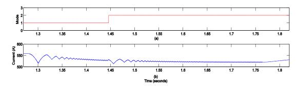
Figure 4.30 Mode detection and change. (a) Operating mode, (b) Reference current.
