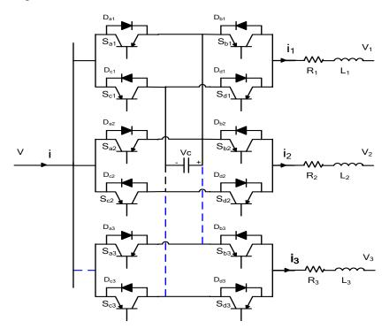
Figure 4.16 Proposed extended three-port CFC topology.
