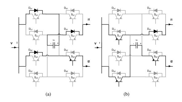
Figure 4.4 CFC operating in mode 1. (a) Charging from cable 1. (a) Discharging in cable 2.
