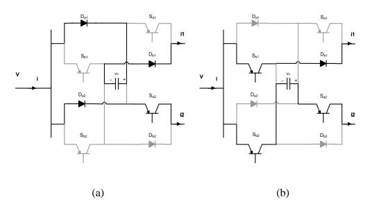
Figure A.29 Reduced switches count topology MCFC operating in mode 1. a) Charging period, b) discharging period.
