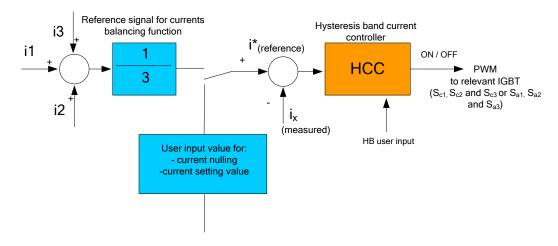
Figure 4.20 Proposed HCC control scheme for the extended 3 ports CFC.
