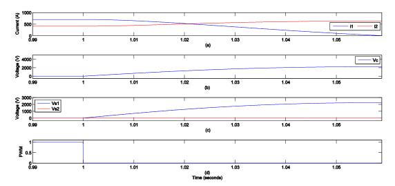
Figure 4.26 Current nulling. (a) Cable currents, (b) Capacitor voltage, (c) Series voltages, (d) PWM signal
