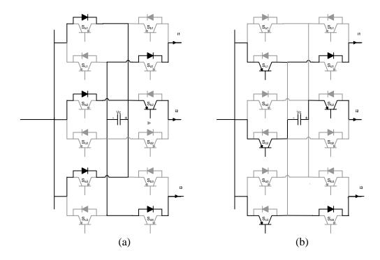
Figure A.10 Extended CFC mode 6 a) Charging from cables 1 and 3, b) Discharging in cable 2.
