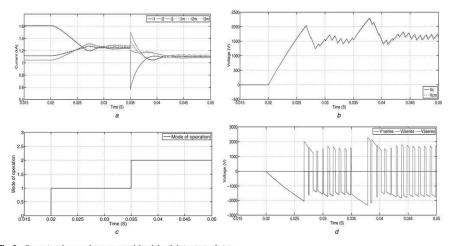
Fig. 8 Comparison between the average model and detailed circuit simulation a Cable currents b Capacitor voltage e Mode of operation d Series voltage introduced to each cable
