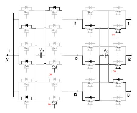
Figure A.27 Three ports MCFC operating in mode 6 - reverse (charging period).
