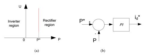
Figure 3.1: Operation in constant power mode a) DC terminal voltage Vs power.
