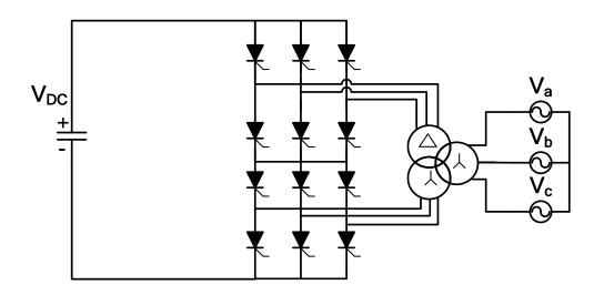
Figure 2.5: 12 pulse Line Commutated Converter circuit topology.
