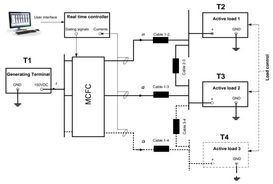
Figure 6.1: Three and four-terminal MTDC grid schematic diagram.
