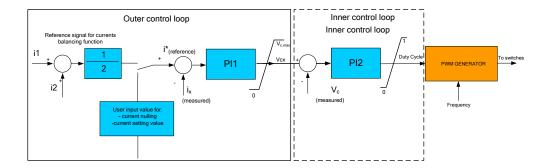
Figure 4.11 Proposed PI controller with capacitor voltage regulation.
