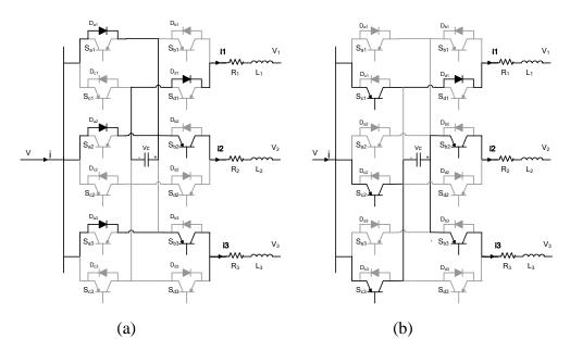
Figure 4.17 CFC extended topology mode 1 a) Charging from cable 1 (mode 1). b) Discharging in cables 2 and 3.
