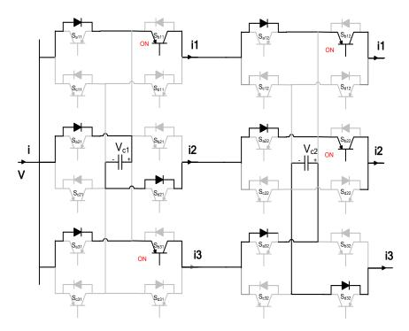
Figure A.19 Three port MCFC operating in mode 2 (charging period).
