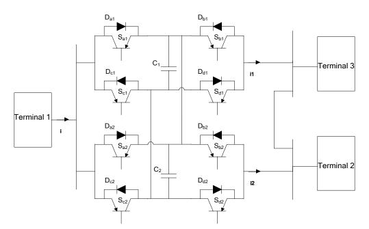
Figure 4.1 Current flow controller preliminary topology.
