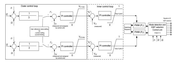
Figure 5.6 Proposed three-port MCFC control loops.
