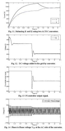
Fig. 13 and Fig.14 show the PI controller output signal and the converter's AC side phase to phase voltage respectively.
