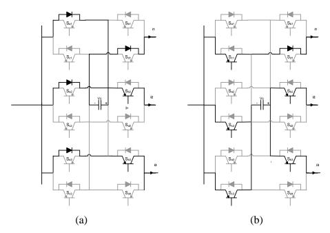
Figure A.5 Extended CFC mode 1. a) Charging from cable 1, b) Discharging in cables 2 and 3.
