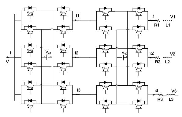
Figure 5.3 Proposed three-port MCFC topology.
