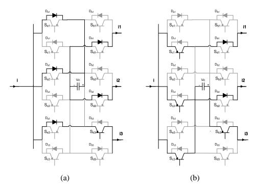
Figure 4.18 CFC extended topology mode 4 a) Charging from cables 1 and 2, b) Discharging in cable 3.
