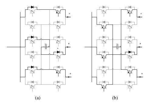
Figure A.6 Extended CFC mode 2 a) Charging from cable 2, b) Discharging in cables 1 and 3.
