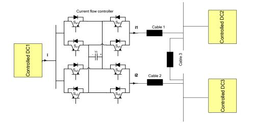
Figure 4.21 Three terminals MTDC grid with 2 ports CFC inserted.
