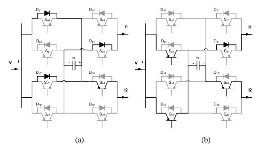
Figure A.1: Two port CFC in mode 1. (a) Charging from cable 1.
