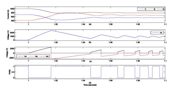
Figure 4.38 Extended CFC unsuccessful balancing (mode 4) - extended topology. (a) Cable currents, (b) Capacitor voltage, (c) Series voltages, (d) PWM signal.
