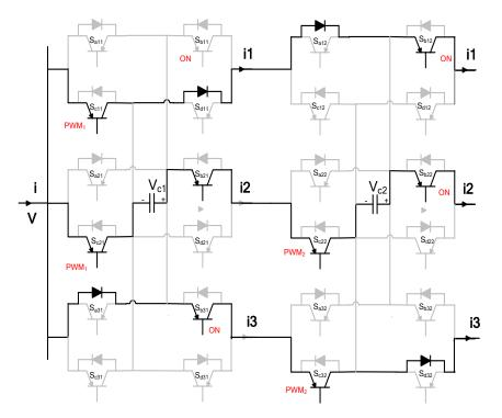
Figure A.22 Three ports MCFC operating in mode 3 (discharging period).
