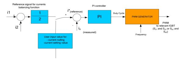
Figure 4.10 Proposed PI controller for CFC.
