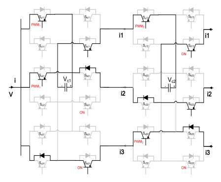
Figure A.26 Three ports MCFC operating in mode 5 - reverse (discharging period).
