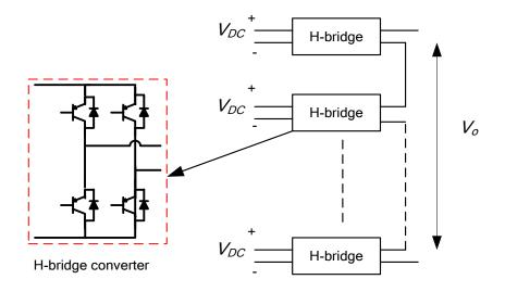
Figure 2.11: H-bridge cascaded multilevel converter.
