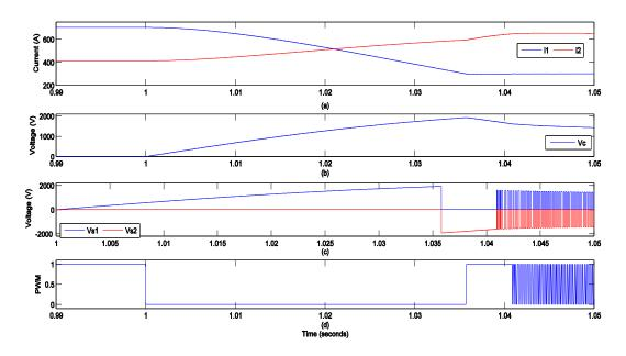
Figure 4.24 Current limiting. (a) Cable currents, (b) Capacitor voltage, (c) Series voltages, (d) PWM signal
