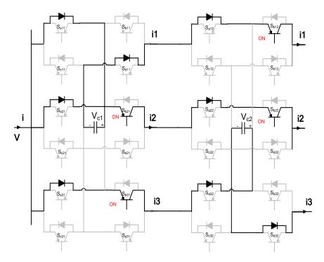
Figure A.21 Three ports MCFC operating in mode 3 (charging period).
