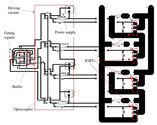
Figure 6.2: MCFC submodule schematic diagram.
