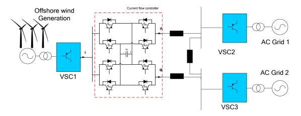
Figure 4.3 CFC inserted in series in a three terminals MTDC grid.
