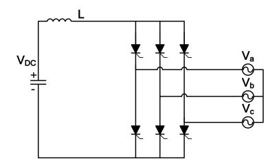
Figure 2.2: Three phase line commutated converter topology.
