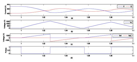
Figure 4.31 Currents balancing with HB=50A. (a) Cable currents, (b) Capacitor voltage, (c) Series voltages, (d) PWM signal.
