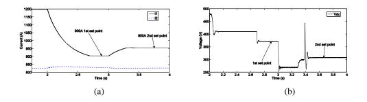
Figure 3.15: a) i1 is set to 900A and 950A using single AC/DC converter.b) DC voltage added to the grid by converter.
