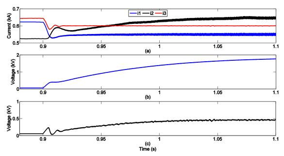
Figure B.13 Setting i1 and i3. (a) Cable currents, (b) Capacitor voltage Vc1, (c) Capacitor voltage Vc2.
