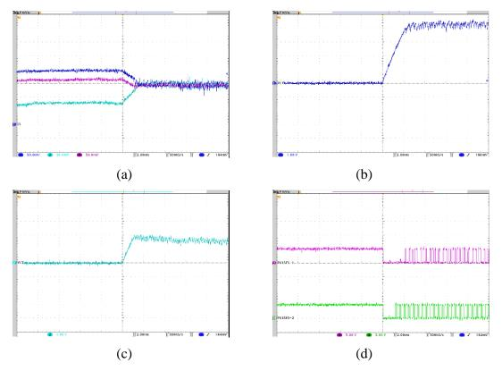
Figure 6.12: Current balancing – three-port MCFC (Y axis: 0.5 A/Div for i1, i2, and i3, 1 V/Div for Vc, and 5 V/Div for PWM, X axis: 2 ms/Div): (a) balanced currents, (b) capacitor voltage Vc1, (c) capacitor voltage Vc2, (d) PWM signals P1 and P2.
