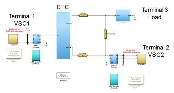
Figure 4.40 VSC based SIMULINK model.
