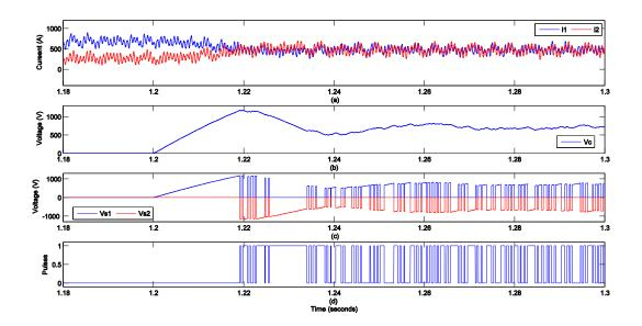
Figure 4.41 VSC based model with CFC currents balancing (mode 1) (a) Cable currents, (b) Capacitor voltage, (c) Series voltages, (d) PWM signal.
