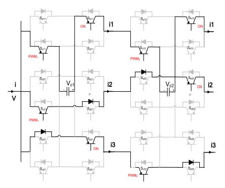
Figure A.20 Three ports MCFC operating in mode 2 (discharging period).
