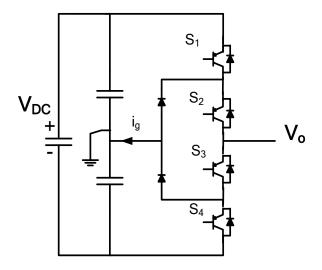
Figure 2.9: Single phase three-level diode clamped converter.
