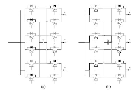
Figure A.16 Extended CFC mode 12 (reverse) a) Charging from cables 1 and 3, b) Discharging in cable 2.
