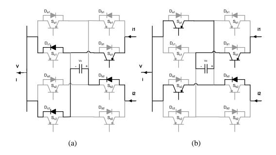
Figure 4.7 CFC operating in mode 4 (reverse). (a) Charging from cable 2. (b) Discharging in cable 1.
