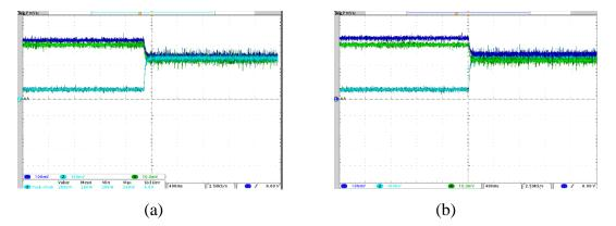
Figure 6.11: Extended topology (Y axis: 1 A/Div for i1, i2 and i3, X axis: 400 ms/Div): (a) low differences in current (b) high differences in current.
