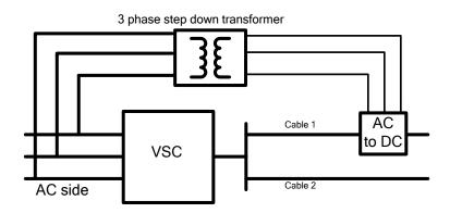
Figure 3.10: AC/DC converter as a power flow controller.
