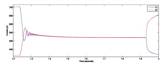
Figure 4.28 Sudden mode change with mode detection unit switched off.
