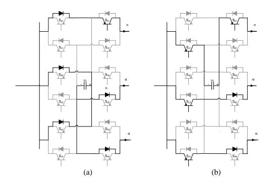
Figure A.9 Extended CFC mode 5 a) Charging from cables 2 and 3, b) Discharging in cable 1.
