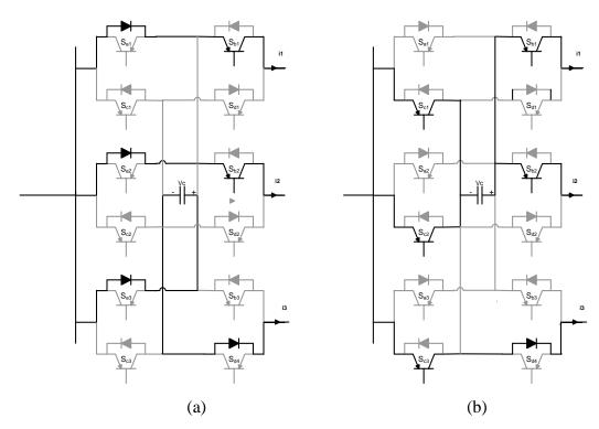
Figure A.7 Extended CFC mode 3 a) Charging from cable 3, b) Discharging in cables 2 and 3.
