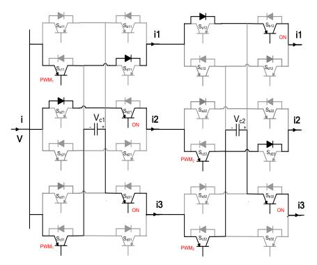
Figure A.18 Three port MCFC operating in mode 1(discharging period).
