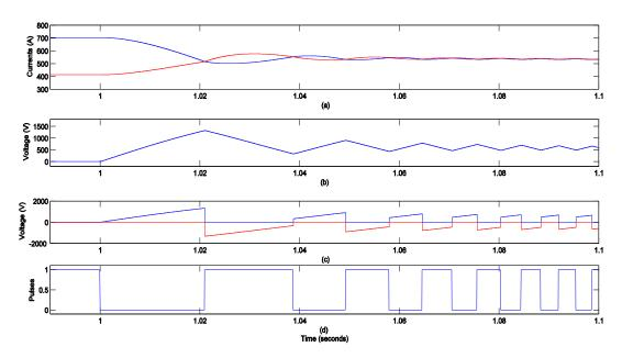
Figure 4.33 Current balancing with HB=0.001A. (a) Cable currents, (b) Capacitor voltage, (c) Series voltages, (d) PWM signal
