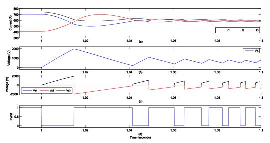
Figure 4.35 Extended CFC currents balancing mode 4 - extended topology. (a) Cable currents, (b) Capacitor voltage, (c) Series voltages, (d) PWM signal.
