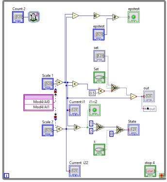
Figure C.4 LABVIEW currents reading and comparing loop.
