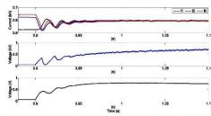
Fig.6. MCFC performing currents balancing: mode 3. a) Cable currents, b) Capacitor voltage Vc1, c) Capacitor voltage Vc2
