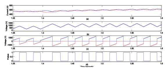
Figure 4.34 Performance under sudden load changes. (a) Cable currents, (b) Capacitor voltage, (c) Series voltages, (d) PWM signal
