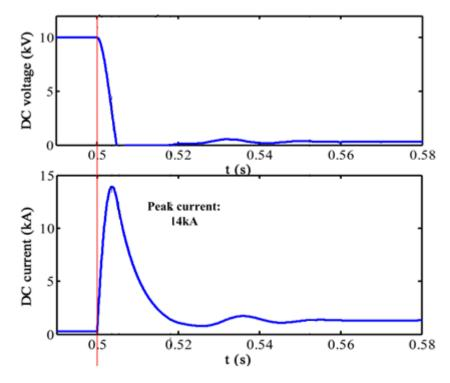
Figure 2.20: DC voltage and current rise during a fault [88].
