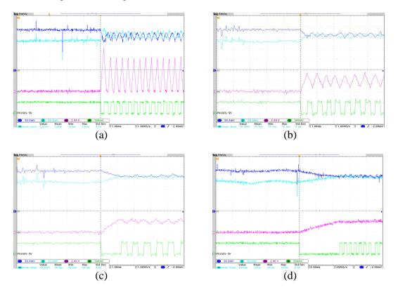
Figure 6.10: Effect of CFC capacitor value (Y axis: 0.5 A/Div for i1 and i2, 2 V/Div for Vc, and 5 V/Div for PWM): (a) CFC capacitor = 47 uF (X axis: 1 ms/Div), (b) CFC capacitor = 220 uF (X axis: 1 ms/Div), (c) CFC capacitor = 1 mF (X axis: 1 ms/Div), (d) CFC capacitor = 9.6 mF (X axis: 4 ms/Div).
