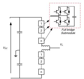
Figure 2.14: Full-bridge modular multilevel converter.
