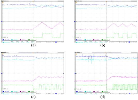
Figure 6.8: Current limiting (Y axis: 0.5 A/Div for i1 and i2, 2 V/Div for Vc, and 5 V/Div for PWM. X axis: 1 ms/Div): (a) balancing currents HB = 150 mA, (b) balancing currents HB = 80 mA, (c) balancing currents HB = 30 mA, (d) balancing currents HB = 5 mA.
