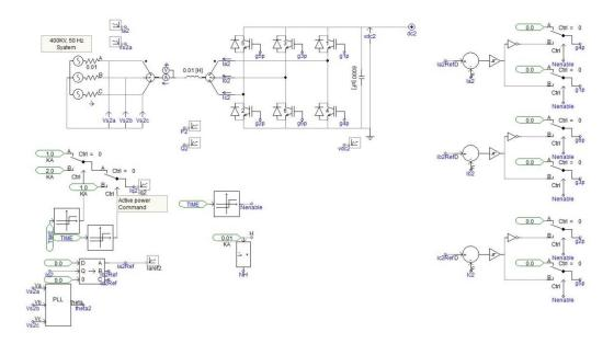
Figure B.10 Converter station 2 control circuit (power control).
