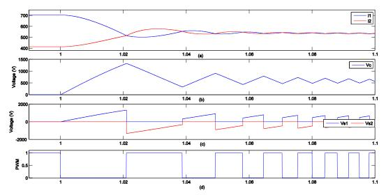
Figure 4.22 Currents balancing. (a) Cable currents, (b) Capacitor voltage, (c) Series voltages, (d) PWM signal
