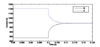
Figure 3.8: Balancing of currents i1 and i2 using series DC voltage sources.
