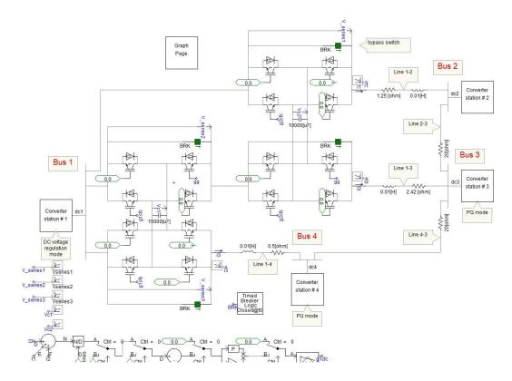
Figure B.8 VSC based four terminals DC grid with MCFC inserted simulation model.
