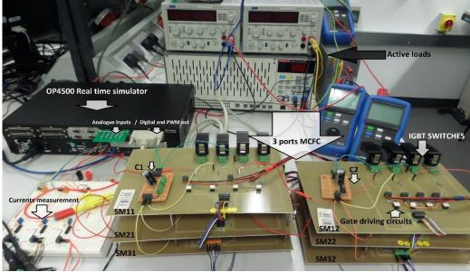
Figure 6.3: MCFC with OP4500 controller experimental setup.
