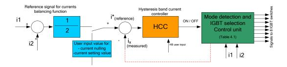
Figure 4.14 Mode detection control unit.
