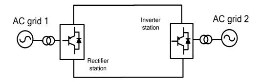
Figure 2.8: Back to back connection using VSC converters.
