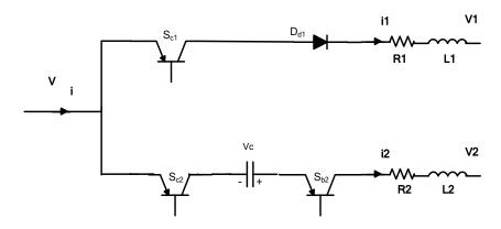
Figure 4.9 CFC circuit during discharging period (mode 1).
