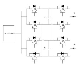
Figure 3.16: Current Flow Controller [13].
