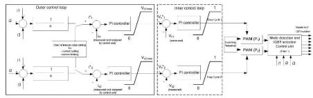
Fig. 5. The proposed control system for the three-port MCFC.
