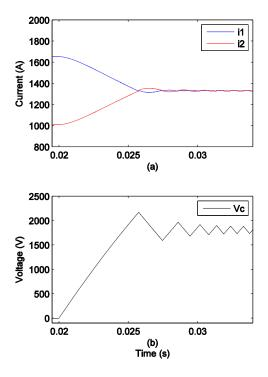
Figure 4.43 Simulation model outputs (a) Cable currents, (b) Capacitor voltage.
