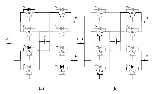
Figure 4.5 CFC operating in mode 2. (a) Charging from cable 2. (b) Discharging in cable 1.
