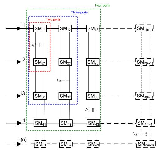
Figure 5.2 Proposed MCFC modular topology for 2, 3, 4, and n ports.
