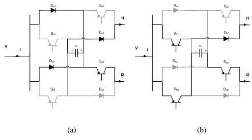
Figure 5.9 Reduced switches count topology MCFC operating in mode 1, (a) charging (b) discharging.
