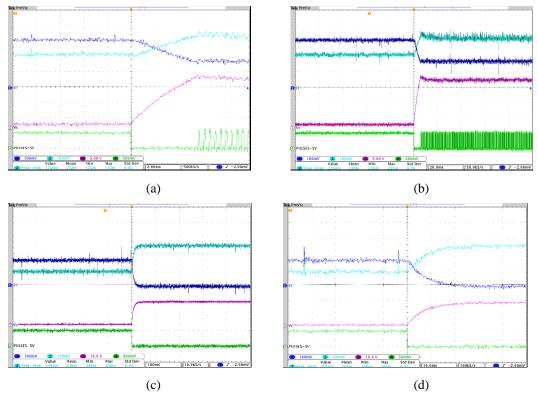
Figure 6.7: Current limiting (Y axis: 1 A/Div for i1 and i2, 5 V/Div and 10 V/Div for Vc, and 5 V/Div for PWM): (a) setting i1 to 1.7 A (X axis: 2 ms/Div), (b) setting i1 to 1.7 A (X axis: 20 ms/Div), (c) nulling i1 (X axis: 100 ms/ Div), (d) Nulling i1 (X axis: 10 ms/Div).
