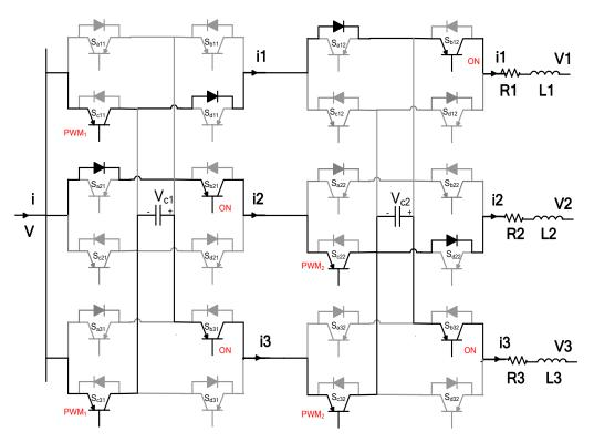
Figure 5.5 Three-port MCFC operating in mode 1(discharging period).
