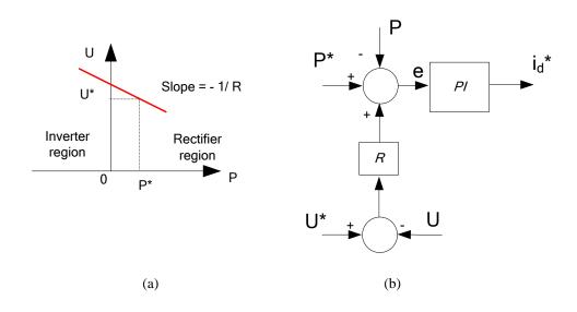
Figure 3.4: voltage droop control a) DC terminal voltage Vs power characteristics. b) Controller schematic.
