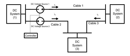
Figure 3.6: Controlled series voltage sources.
