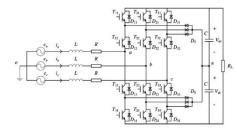
Fig. 6. Typical 3 level AC/DC converter circuit topology [11].
