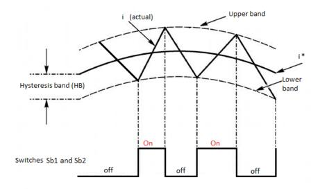
Figure 4.13 Hysteresis band current controller operation.
