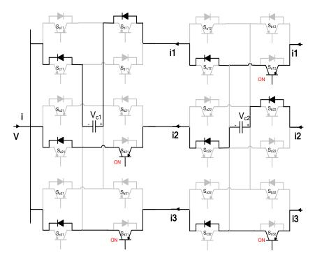
Figure A.23 Three ports MCFC operating in mode 4 - reverse (charging period).
