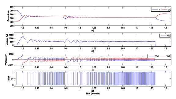
Figure 4.29 Mode detection and change. (a) Cable currents, (b) Capacitor voltage, (c) Series voltages, (d) PWM signal
