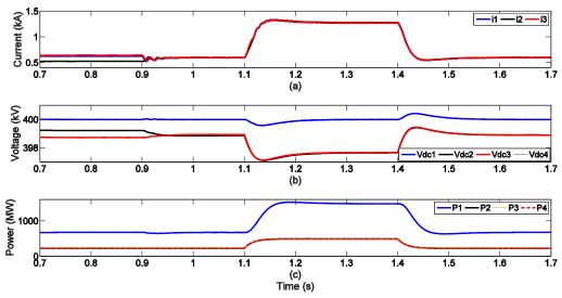
Figure B.12 Dynamic performance of MCFC under sudden load change. (a) Cable currents, (b) Terminal voltages, (c) Active powers.
