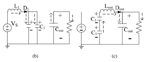
Figure 2.21: Marx DC/DC converter a) Circuit topology b) Charging period c) Discharging period [95].
