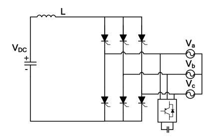
Figure 2.4: Active filter connected to LCC-HVDC system.
