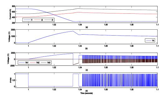
Figure 4.37 Extended CFC limiting i1 to 250A (mode 1) - extended topology. (a) Cable currents, (b) Capacitor voltage, (c) Series voltages, (d) PWM signal.
