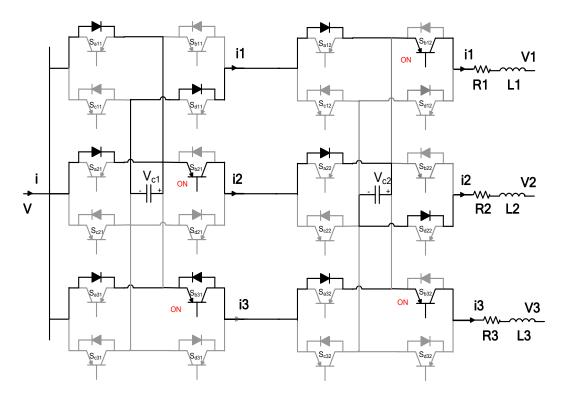
Figure 5.4 Three-port MCFC operating in mode 1(charging period).
