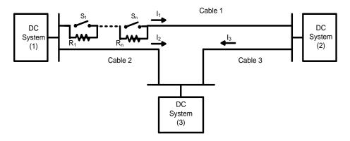
Figure 3.5: Switching series resistors.
