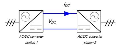
Figure 2.17: Back to back HVDC connection.
