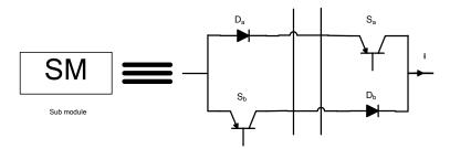
Figure 5.7 Building block of the reduced switches count MCFC.
