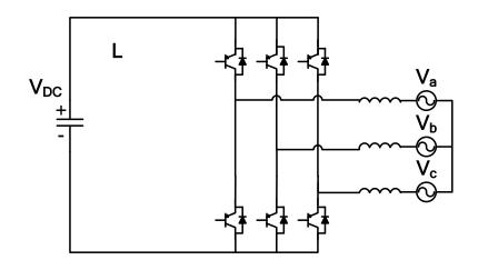
Figure 2.7: Three phase two level self-commutated – Voltage Source Converter (VSC).
