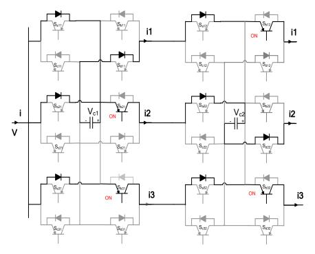
Figure A.17 Three port MCFC operating in mode 1(charging period).
