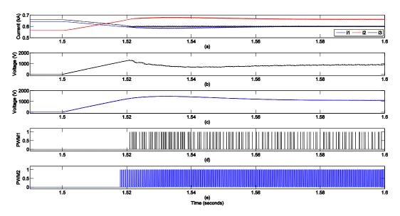
Figure 5.12 MCFC currents  $i_1$  and  $i_3$  setting. (a) Cable currents, (b) Capacitor voltage  $V_{c1}$ , (c) Capacitor voltage  $V_{c2}$ , (d) PWM<sub>1</sub> signal, (e) PWM<sub>2</sub> signal
