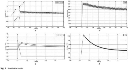
a Cable currents during balancing b Capacitor voltage during balancing c Cable currents during current setting d Capacitor voltage during current setting
