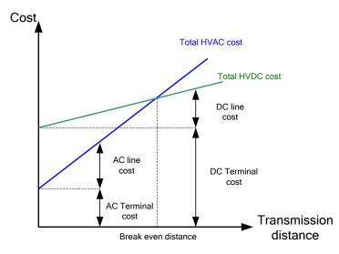
Figure 2.1: Power transmission cost versus distance with both HVDC and HVAC solutions.
