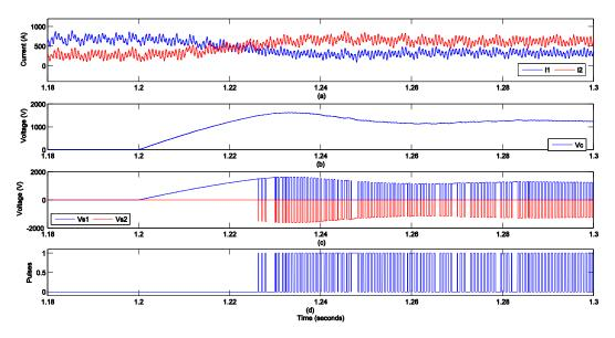
Figure 4.42 VSC based model with CFC currents limiting (mode 1) (a) Cable currents, (b) Capacitor voltage, (c) Series voltages, (d) PWM signal.
