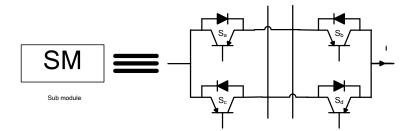
Figure 5.1 Building block of the MCFC.
