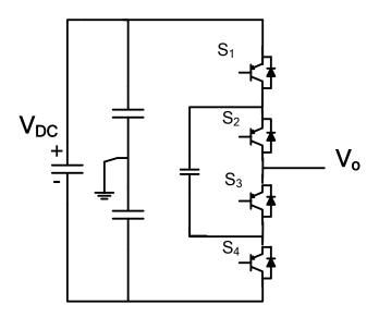
Figure 2.10: Single phase three-level flying capacitor converter.
