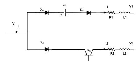
Figure 4.8 C circuit during charging period (mode 1).
