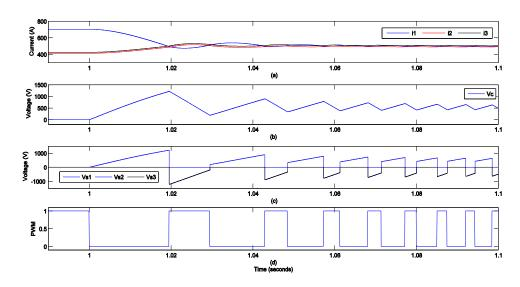
Figure 4.36 Extended CFC currents balancing mode 1 - extended topology. (a) Cable currents, (b) Capacitor voltage, (c) Series voltages, (d) PWM signal.
