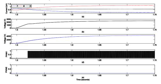
Figure 5.13 MCFC nulling  $i_3$  and setting  $i_1$ . (a) Cable currents, (b) Capacitor voltage  $V_{c1}$ , (c) Capacitor voltage  $V_{c2}$ , (d) PWM<sub>1</sub> signal, (e) PWM<sub>2</sub> signal
