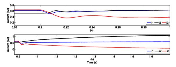
Figure B.14 MCFC performing simultaneous tasks. (a) Setting i3 to 0.375kA and balancing i1 and i2, (b) Nulling i3 and setting i1 to 0.6kA.
