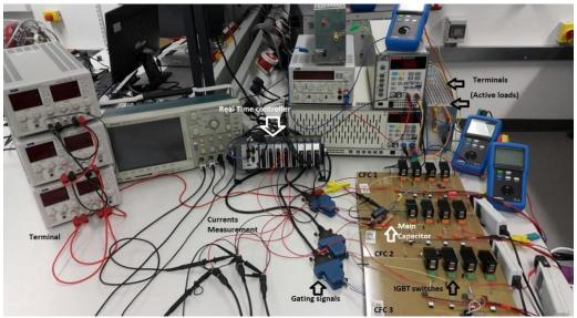
Figure 6.4: Extended topology CFC with NI-Crio controller experimental setup.
