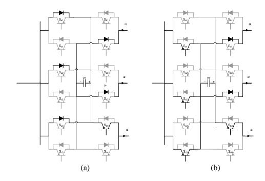
Figure A.8 Extended CFC mode 4 a) Charging from cables 1 and 2, b) Discharging in cable 3.
