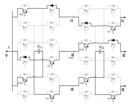
Figure A.24 Three ports MCFC operating in mode 4 - reverse (discharging period).
