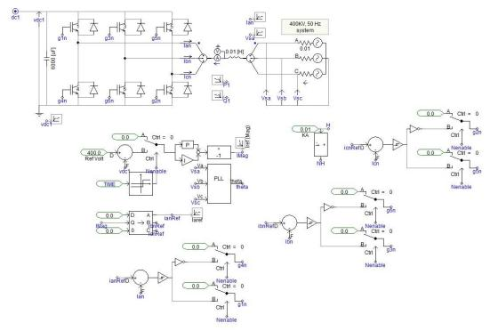
Figure B.9 Converter station 1 control circuits (voltage regulating).
