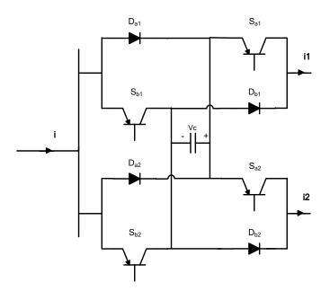
Figure 5.8 Reduced switches count topology of two-port MCFC.
