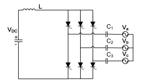
Figure 2.6: Circuit topology of Capacitor Commutated Converter (CCC).
