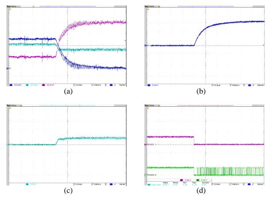
Figure 6.13: Setting i2 and nulling i1 – MCFC (Y axis: 0.5 A/Div for i1, i2, and i3, 5 V/Div for Vc, and 5 V/Div for PWM, X axis: 10 ms/Div): (a) cable currents, (b) capacitor voltage Vc1, (c) capacitor voltage Vc2, (d) PWM signals P1 and P2.
