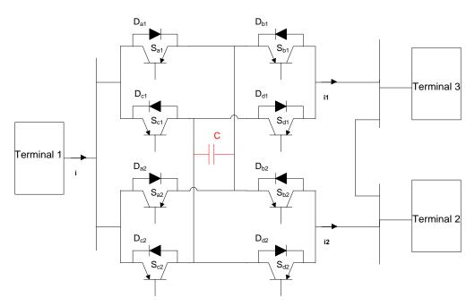
Figure 4.2 Current flow controller with single capacitor.
