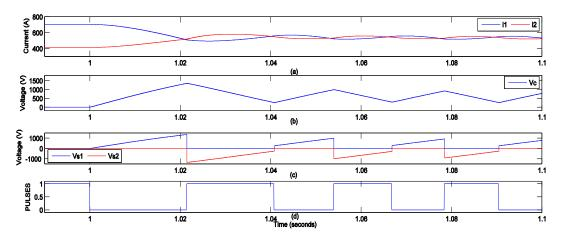
Figure 4.32 Current balancing with HB=5A. (a) Cable currents, (b) Capacitor voltage, (c) Series voltages, (d) PWM signal
