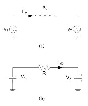
Figure 2.22: Basic electrical connection. a) AC circuit b) DC circuit.
