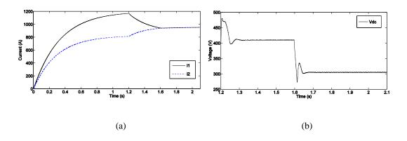
Figure 3.12: a) Balancing *i*<sub>1</sub> and *i*<sub>2</sub> using two AC/DC converters.(b) DC voltage added to the grid by converter.
