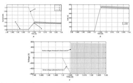
Fig. 6 Charging the capacitor from cable 1 and discharging in cables 2 and 3 a Cable currents b Capacitor voltage c Series voltages
