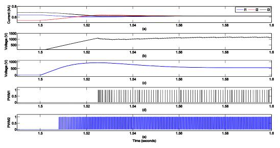
Figure 5.10 MCFC currents balancing - mode 3. (a) Cable currents, (b) Capacitor voltage  $V_{c1}$ , (c) Capacitor voltage  $V_{c2}$ , (d) PWM<sub>1</sub> signal, (e) PWM<sub>2</sub> signal
