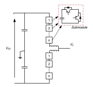
Figure 2.13: Half-bridge modular multilevel converter.
