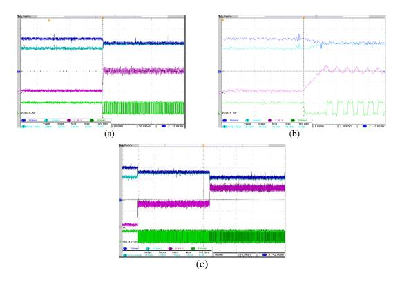
Figure 6.6: Current balancing (Y axis: 1 A/Div for i1 and i2, 2 V/Div for Vc, and 5 V/Div for PWM): (a) balancing i1 into i2 (X axis: 20 ms/Div), (b) balancing i1 into i2 (X axis: 1 ms/Div), (c) sudden load change (X axis: 100 ms/Div).
