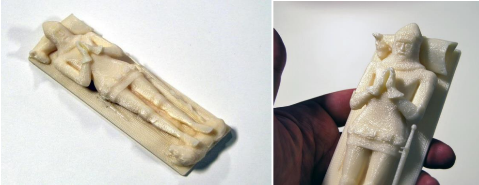
Figure 20: Final 3D print after removal of the support material.
