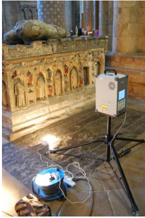
Figure 3: The Minolta 3D Scanner used to scan the surface topology of the tomb of Sir John Neville
