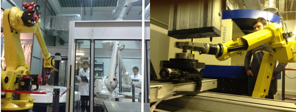
Fig 2. The 3.05m and 2.55m robots (left), and the 1.8m robot and Zeeko IRP600 machine in Automation Cell (right)
