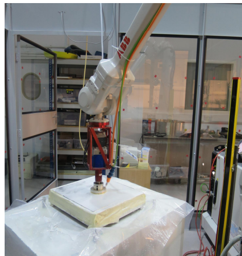
Figure 3. Grolishing experiment on glass bending equipment.
