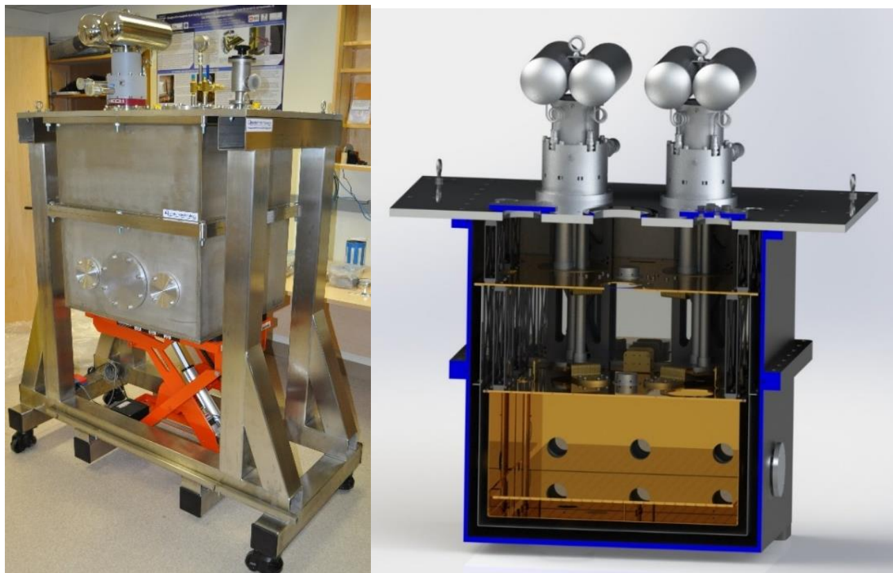
Figure 2. (Left) The TFC after delivery to the University of Lethbridge. A single PTC can be seen on the top plate. The horizontal split in the vacuum chamber allows for the bottom half of the chamber to be lowered by the scissor jack. Three blank flanges for the side apertures are also shown. (Right) A cross sectional view of the TFC. The dual pulse tube arrangement, CFRP supports, and rectangular, paneled shields are shown.
