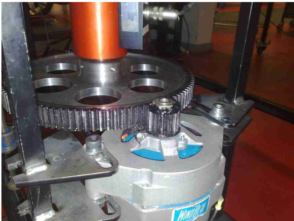
Figure 4.2: Torque transducer, gear train and generator
