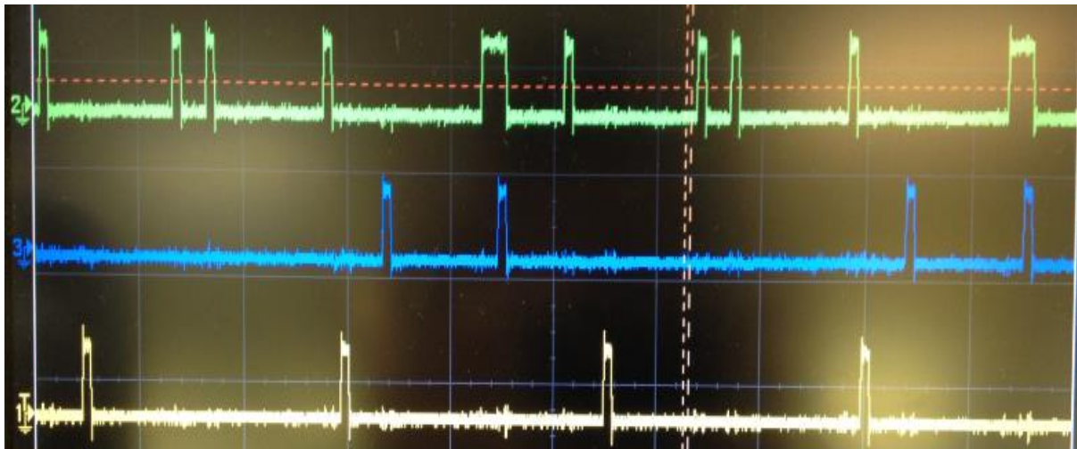
Fig. 8.11: Experimental verification of all three error flags for invalid sequences: wrong-slot flag (top trace), erasure flag (middle trace) and false-alarm flag (bottom trace).
