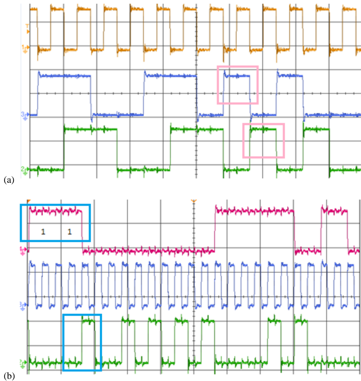
Fig. 7.8 (a) and (b): Experimental results of duobinary PPM coder (a) top trace is the PCM clock and bottom trace is one clock cycle shifted PCM data (middle trace) and (b) bottom trace is the coded duobinary PPM data. PCM data (Top trace) and clock (middle trace)
