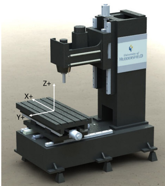
Fig. 2. Three-axis machine tool.
