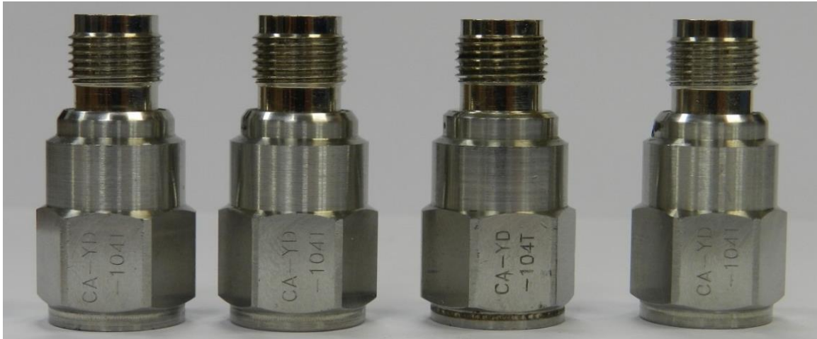
Figure 8-13: Photograph of four accelerometers (model CA-YD-104T)
