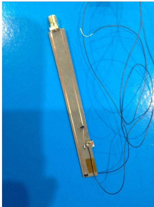
Fig. 34 The matching network chip consisting of microstrip phase shifters and the low-pass filter
