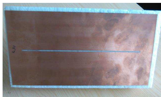
Fig.23 Copper etched slot antenna
