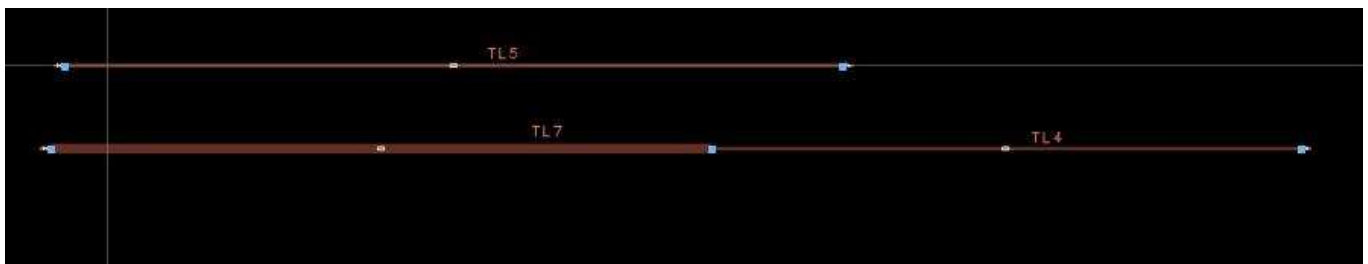
Fig. 22 Realisation of microstrips in the layout using RO3010 duroid substrate
