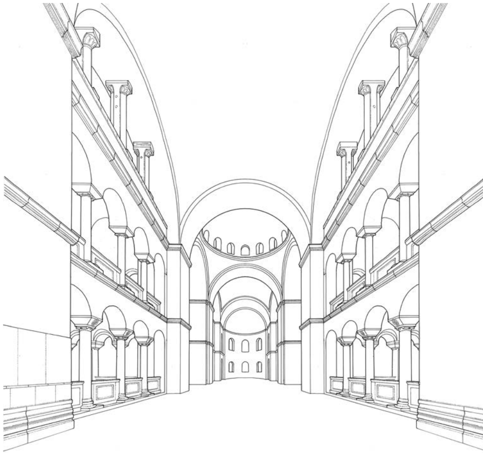
FIG. 7.11. Reconstruction of the church of St. John in Ephesus, perspective view of the interior, looking east. Notice the “thermal” windows at the top of the lateral screens (drawing by author, 2013).
