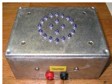
Figure 1: The emitter part of the optical identification sensor
