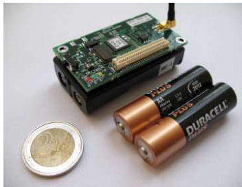
Figure 7: MPR2400 MICAz mote
