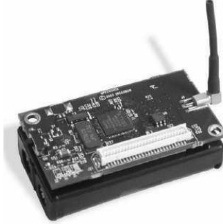
Fig. 7. MICAz mote used for localisation sensor
