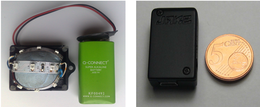
Fig. 1. (a) IR tag with 9V battery attached, (b) JAKE sensor pack shown with a five cent euro piece. Image provided courtesy of Stephen Hughes.
