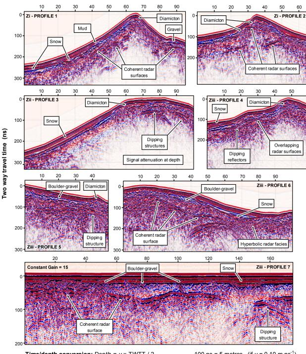
**Time/depth conversion:** Depth =  $v \times TWTT / 2$ AGC applied to all profiles (unless stated)
