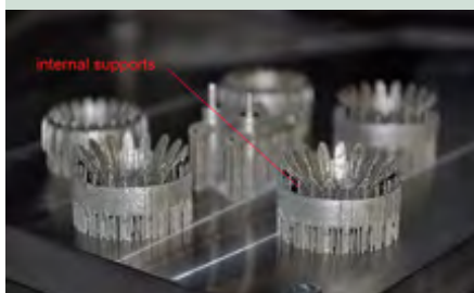
Figures 5(L) & 6(R) showing working prototypes with internal scaffolds and final design, produced without internal supports ©Niedderer 2015
