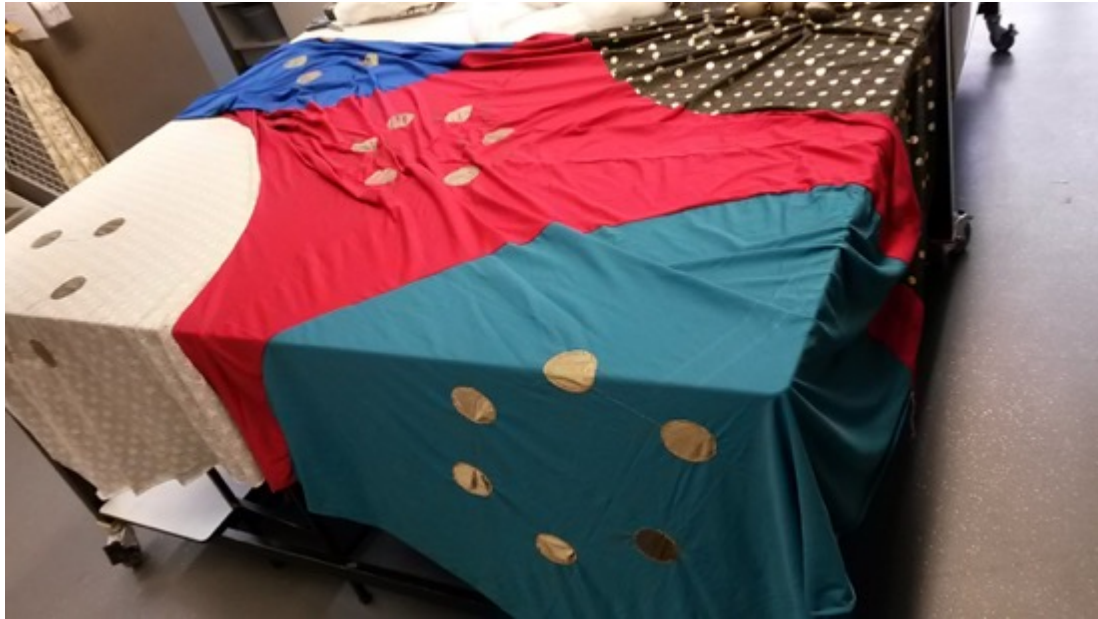
Figure 4. Capacitive ball rug in development, showing the five panels pieces together with the applied conductive fabric.
