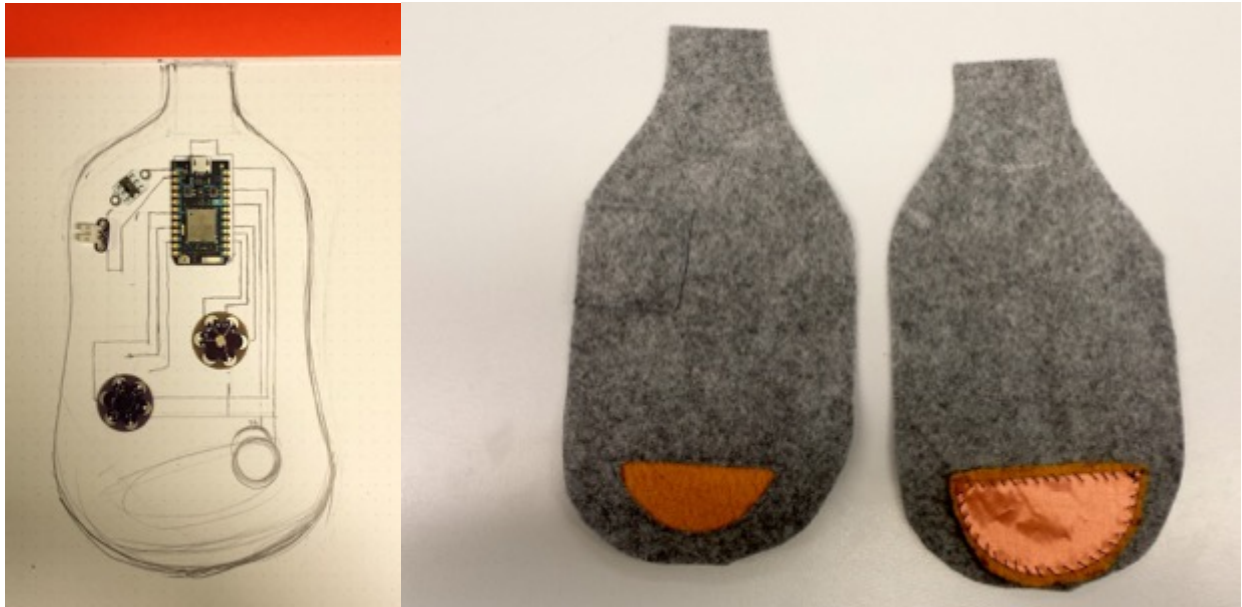
Figure 3. Images of one of the hand-held objects using an accelerometer, on/off switch, push button and a three colour LEDs Lilypad board with a Photon board for wireless communication. Preparatory circuit sketch and intermediary object.
