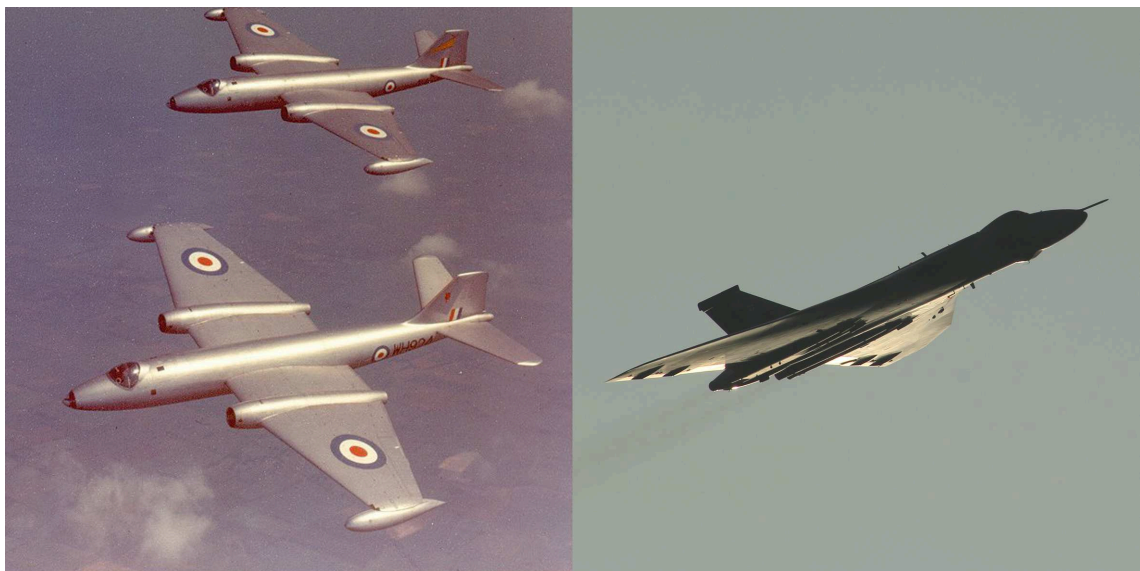
Figure 2.2 Left: English Electric Canberra, courtesy of RAF (Crown Copyright) Right: A Vulcan aircraft over Wilstead, Bedfordshire, courtesy of Mr P. Marlton. The two aircraft are very different in both shape and size, the Canberra has a wing area of 89 m 2 and the Vulcan has a wing area of 368 m 2 .
