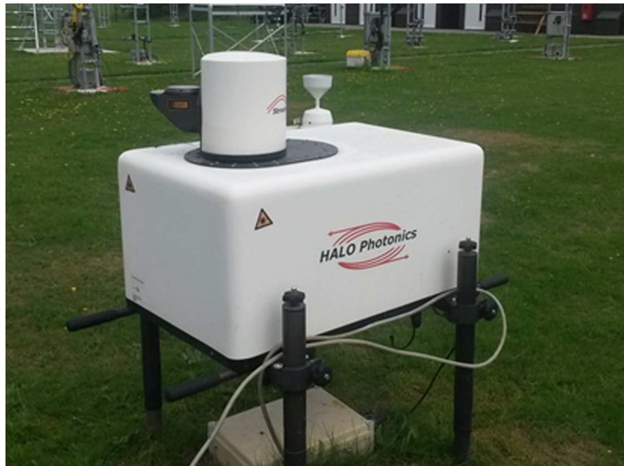
Figure 2.7 A pulsed Doppler lidar at the Reading University Atmospheric Observatory.
