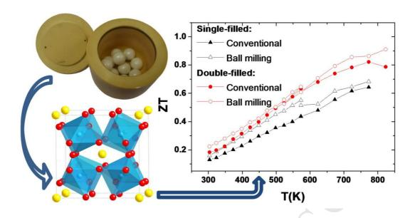
Enhancing the thermoelectric properties of single and double filled p-type skutterudites synthesized by an up-scaled ball-milling process
