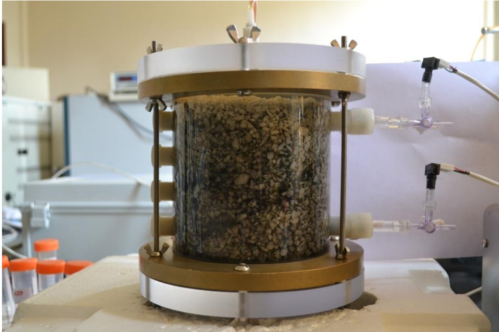
Fig. 1. Black FeS coatings formed in situ on limestone in column experiments. The FeS in the photo was generated by successively injecting SRB and JF-5 bacterial solutions and ageing the mixture for 6 days.
