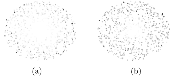
Figure 8 Energy map for LEACH protocol: (a) without charger and (b) with charger
