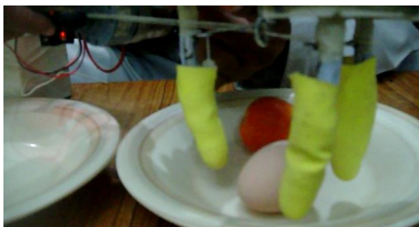
Fig. 10. Experiments with the developed gripper having three soft fingers. Grasping, picking and placing of the raw egg are demonstrated.
