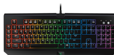
Figure 1: A keyboard with individual backlit LEDs under each key
