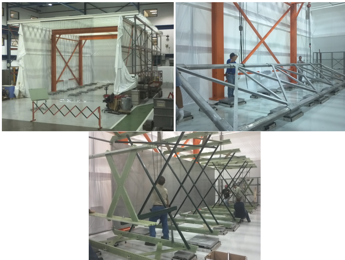
Figure 22. Top Left: Clean tent where MicroBooNE LArTPC assembly was conducted. Top Right: Anode frame in the process of being moved from the metal assembly platforms. Bottom: Cathode frame and G-10 ribs on metal assembly platforms.
