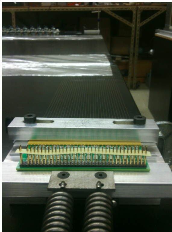
Figure 20. Photograph of a collection plane wire carrier board on the tension stand.
