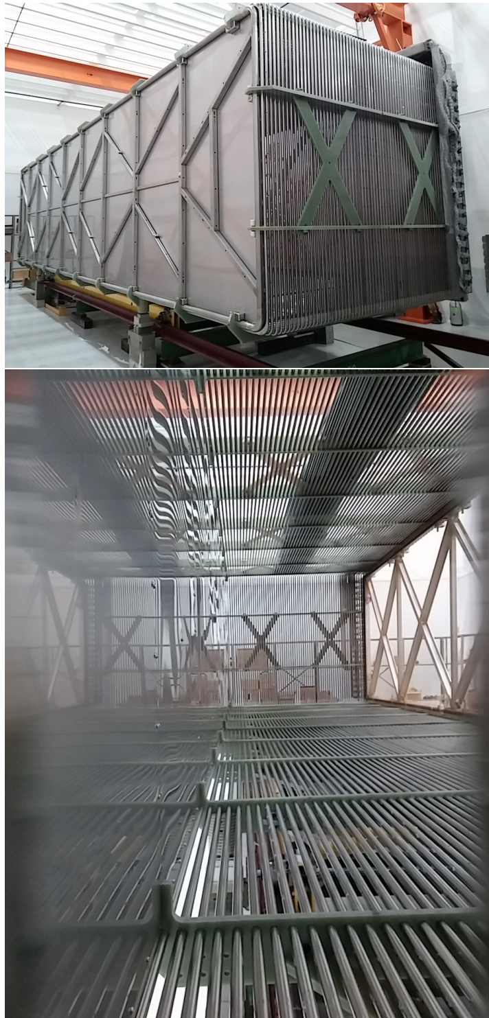
Figure 10. Top: Exterior view showing the cathode frame and structural supports to which cathode sheets are fastened. Bottom: Interior view of cathode plane as viewed from the upstream end of the LArTPC , showing cathode sheets. Note that the cathode sheets are polished, so a reflection is is clearly present in this photograph.
