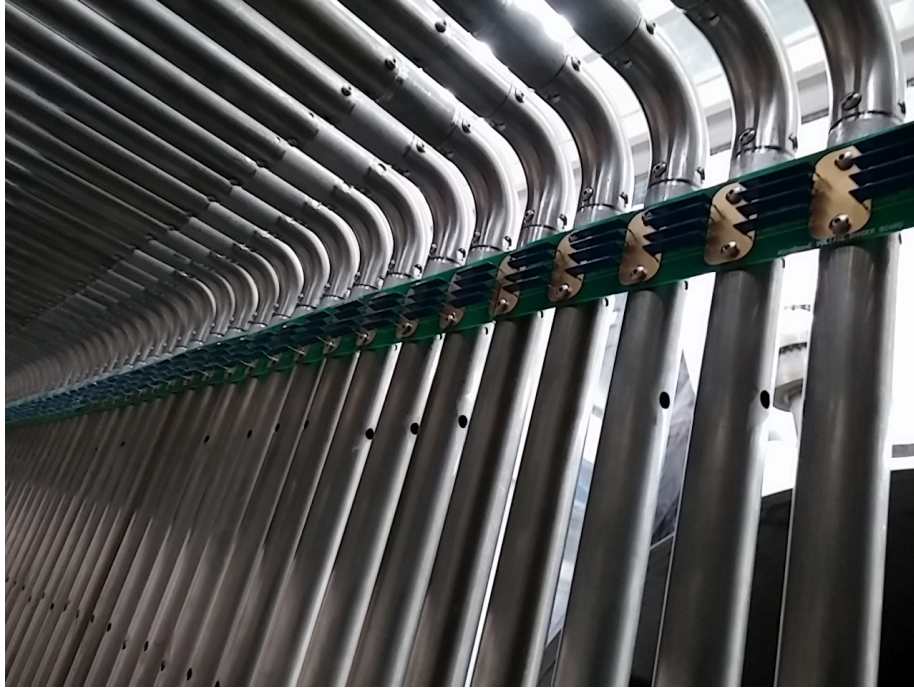
Figure 14. The Ohmite Slim-Mox 104E resistors arranged in parallel sets of four on printed circuit boards that span eight field cage tubes.
