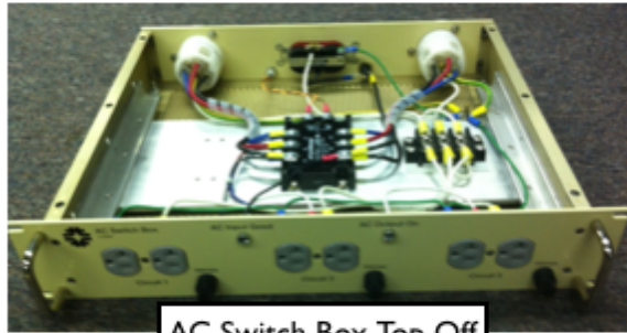
AC Switch Box, Top Off
