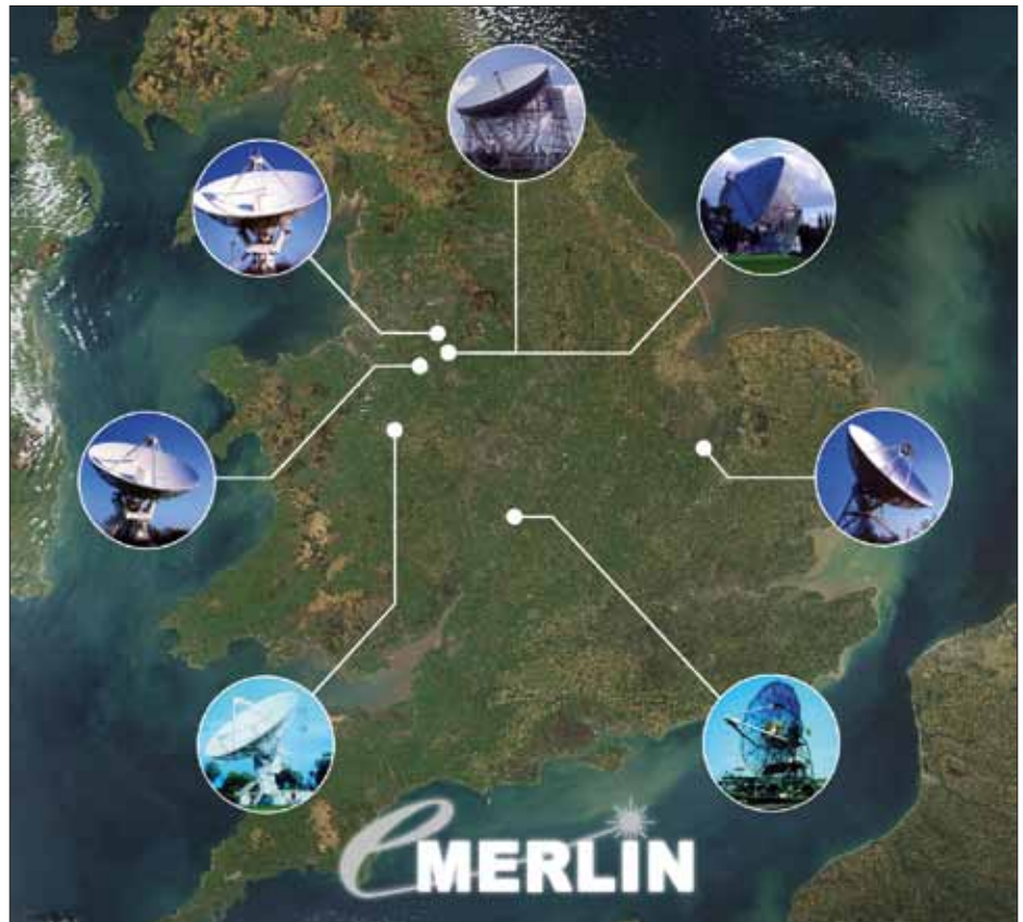
1 The locations of the e-MERLIN telescopes. Clockwise from top: Jodrell Bank Lovell, Jodrell Bank Mk2, Cambridge, Defford, Knockin, Darnhall and Pickmere. Linking them boosts the resolution, and optical fibre connections to increase the bandwidth enhance the sensitivity. (S Lowe/JBCA, Univ. Manchester)
