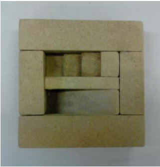
Fig. 14. Photograph of the machined MDF sample showing step and wedge defects.
