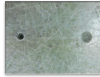
Fig. 17. Photograph of the GFRP sample showing two machined circular defects of 2 mm and 4 mm diameters.
