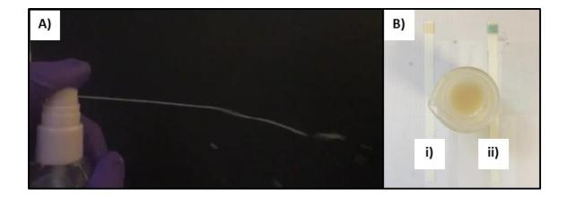
**Fig. 4.** (A) Surgihoney<sup>™</sup>RO<sup>®</sup> spray and (B) hydrogen peroxide test strips demonstrating no detectable concentration of peroxides before water addition (i) and production of ca. 3–10 ppm of detectable peroxides after water addition (ii).
