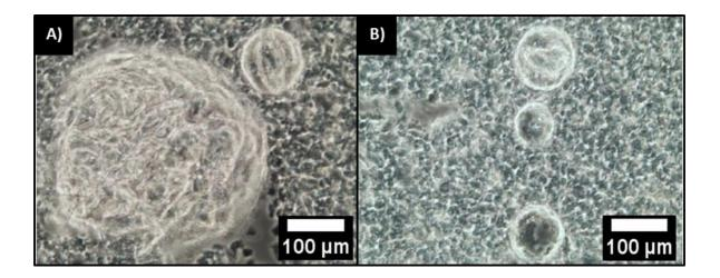
**Fig. 3.** Micrographs of successful reverse micelles containing Surgihoney<sup>™</sup>RO<sup>®</sup> in a continuous phase of paraffin oil demonstrating the presence of (A) coalesced droplets and (B) smaller stable individual droplets.
