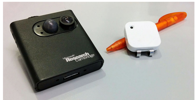
Figure 1: Left: Microsoft SenseCam; Right: Narrative Clip 1.
