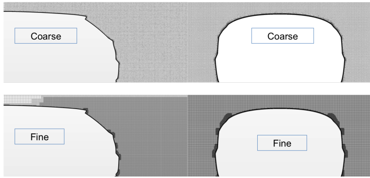
Figure 5: Slices through the symmetry plane of the meshes used for the DES calculations (estate configuration)
