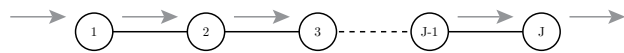
Figure 3 (Above) A linear network with J links. Each packet must pass through each link.
