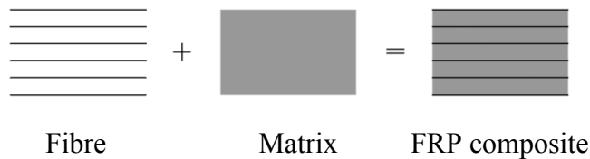
Figure 1-1 FRP composition from fibre and matrix based on Mazumdar(2002)
