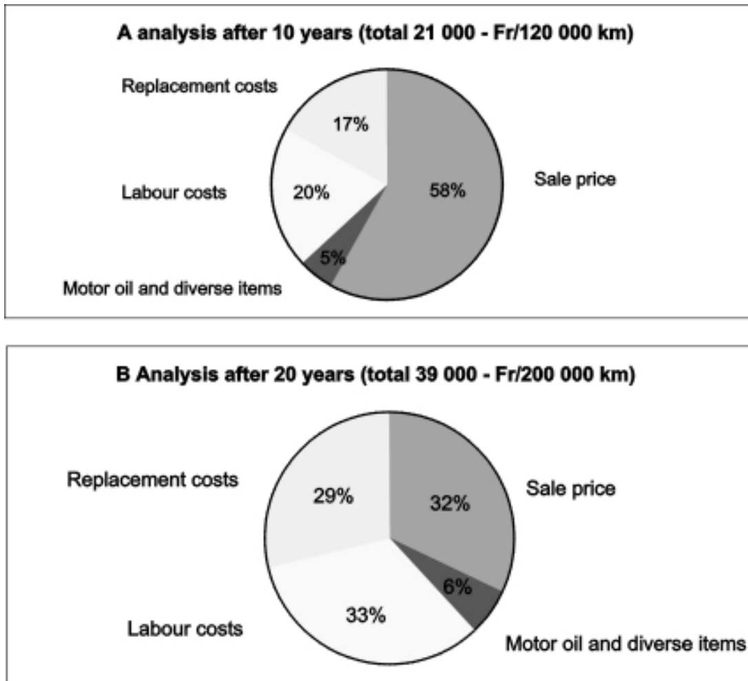
Figure 2.2. Comparison of energy and labour input for manufacturing and maintenance of a middle class car (Toyota Corina MK II, 1969) with a utilisation period of 10 and 20 years; without gasoline
