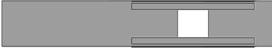
Figure 3.3 CFRP locations at opening of the beam.
