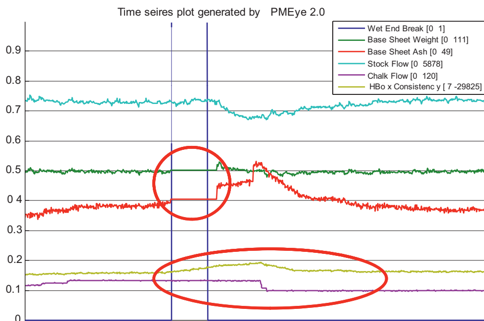
Fig. 4. The Wet End Break is shown by the thick blue line. When the break occurs, the Base Sheet Ash reading freezes. The DCS system is blind to the rising value of the Headbox Ash which is reflected in the bump in the Headbox consistency value after the break.
