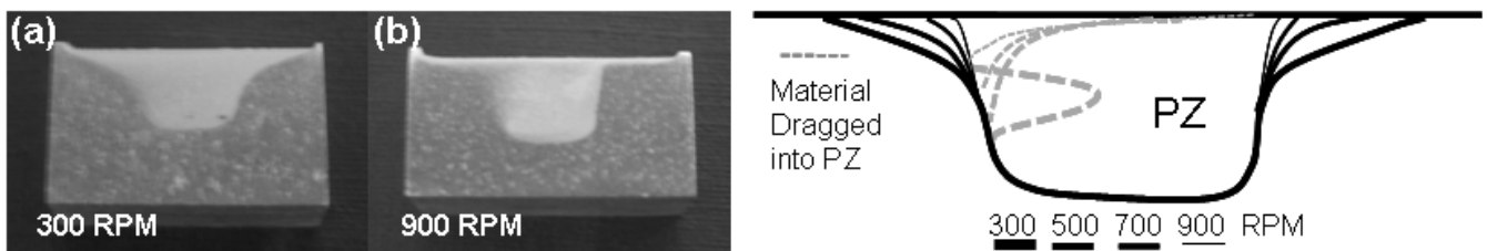
Fig. 5: Profiles of the PZ shown in example macrographs (a) and (b) and mapped in (c) following FSP at 200 \text{ mm min}^{-1} with increasing tool RPM.
