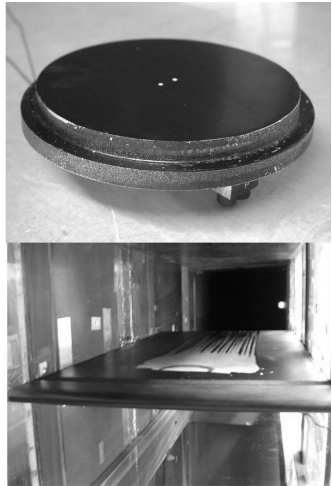
Figure 1. Illustration of small-scale synthetic actuator zero pressure gradient turbulent boundary layer rig. Clockwise from left: Exploded view of one actuator; two such actuators mounted in the circular plate; Circular plate assembly mounted in the flat-plate aerofoil, and in the 0.5m \times 0.5m Goldstein tunnel.
