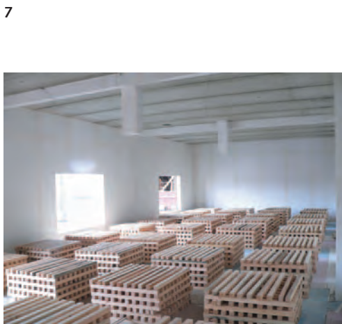
Fig 5. Geometry and strand location of the units / Fig 6. Vertical static load applied using 60 (1t) sandbags / Fig 7. Wooden cribs used for the fire load / Fig 8. Locations of vertical and horizontal measurements
