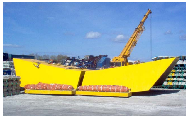
Figure 4. Porch units for concrete protection cover stored in yard; higher ends abut opening in Figure 3 when installed on the seabed.
