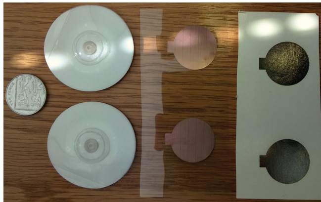
Fig. 1. ECG electrodes with a UK 10p piece for scale. (Left) Traditional Ag/AgCl ECG electrodes. (Middle) Copper printed capacitive electrodes. (Right) Silver printed electrodes on tattoo paper.
