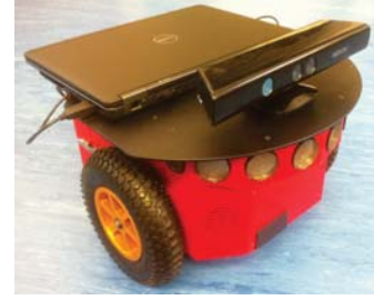
Figure 14. Microsoft Kinect mounted on Pioneer P3-DX mobile robot.
