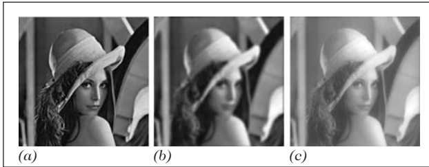
Figure 7. Simulation of the image degradation due to aberrations and scattering. (a) Original image; (b) blurred image; (c) degradation due to straylight only.
